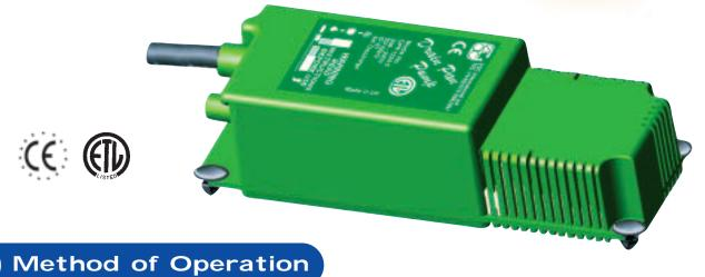
The DPP Drain Pan Pump contains proven electronic water detectors and a pump which turns on to remove the defrost water from a refrigeration cabinet, or condensate water from an air conditioner or condensate boiler.
